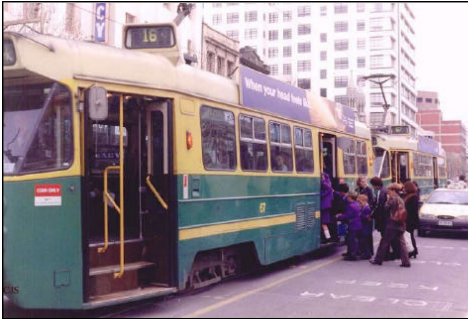
FIGURE 3: Example Kerbside Loading Tram Stop – Down Stream Road Traffic Must Wait for Passenger Boarding and Alighting
