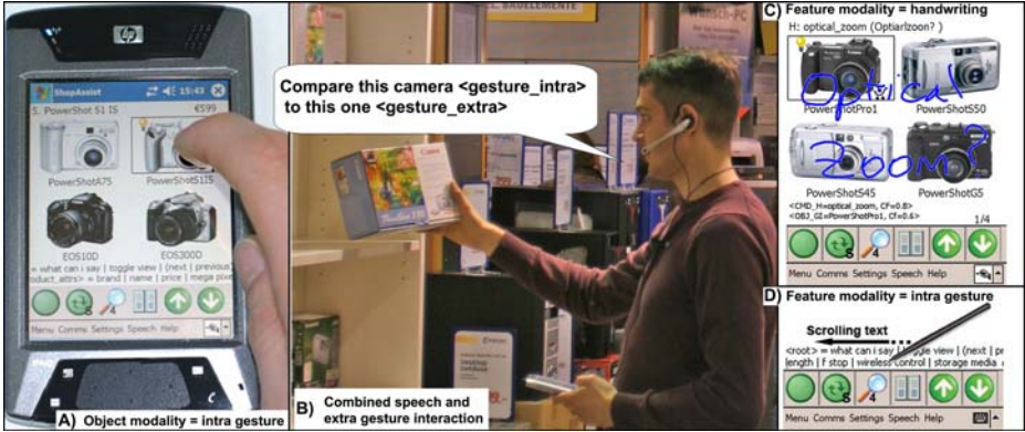
Fig. 1. A and B show the combined use of speech, intra- and extra-gesture. C shows feature selection via handwriting, while D shows feature selection via an intra-gesture point on the scrolling text bar
