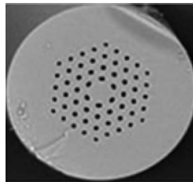
Fig. 1. Silica MOF having a typical hexagonal arrangement of holes (photograph courtesy of the Optical Fibre Technology Centre).
