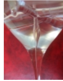
Fig. 7. Neck-down region of an extending PMMA preform containing a centrally located hole.
