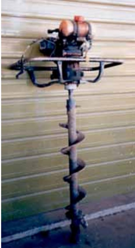
**Portable engine-driven posthole digger**
