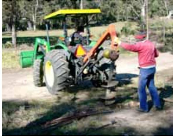
**The worker standing behind the digger is in danger of being struck and/or entangled if the auger hits an object and jumps from the hole. Wire, steel posts and tools lying near the posthole increase the hazard.**
