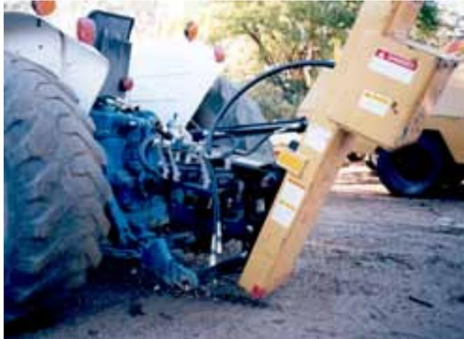
**Three-point-linkage mounted post driver.**
