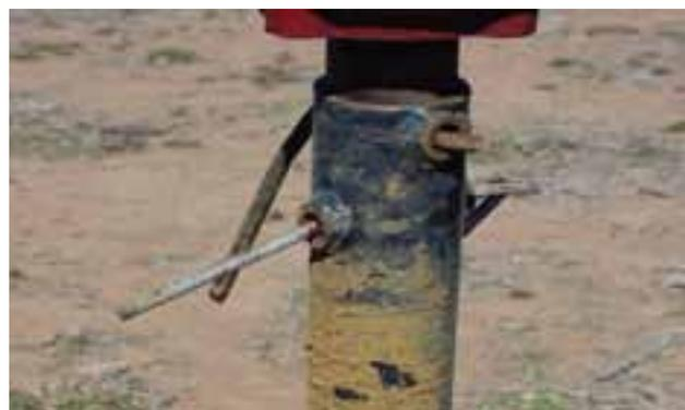
**Picture showing shear pins replaced with steel rods. The protruding ends make this very dangerous.**
