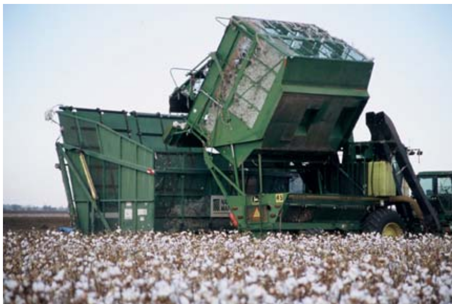
Figure 5.6: Emptying modern picker. Photo courtesy Cotton Australia website
