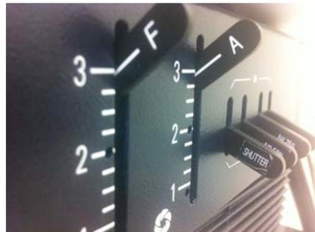
3. When ready for confocal imaging, pull **lever from in to out** (top left of microscope) and make sure FL shutter closed and BF position (5) selected on filter turret.
