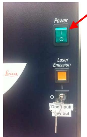
3. Switch on Microscope (if needed for BF). Green switch on left hand side of microscope.
