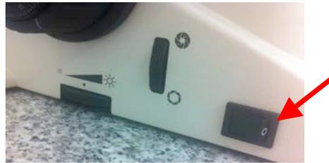
4. Switch on EL6000 fluorescent lamp if using fluorescent samples. Shutter is always open and note position of attenuator. Can open this fully or close down if bright.
