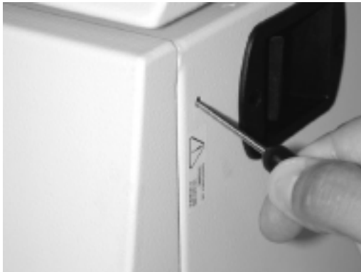
Insert the unlocking tool horizontally into the hole on the right hand side of the instrument.
