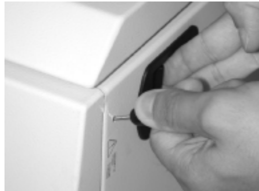
While pressing up with your finger, to press down with the unlocking tool, pull the lid lever toward you: the lid opens upwards.
