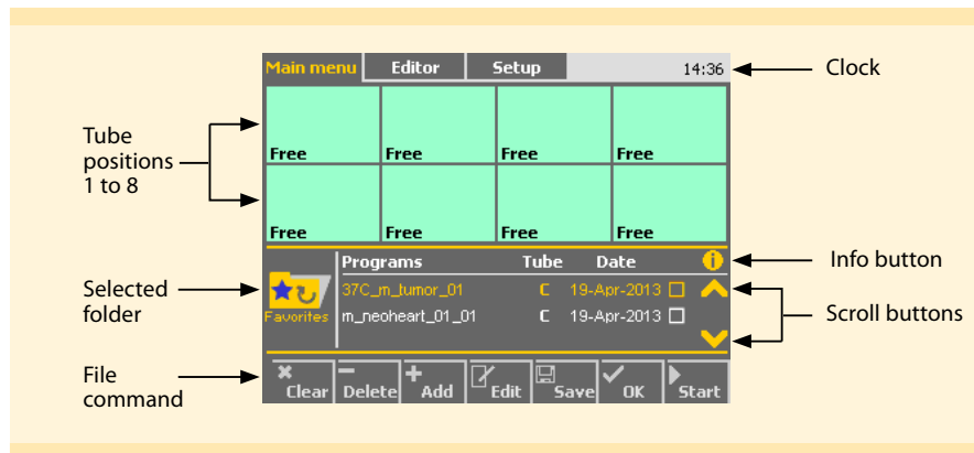
Figure 4.4: Main menu of the gentleMACS Octo Dissociator with Heaters.
