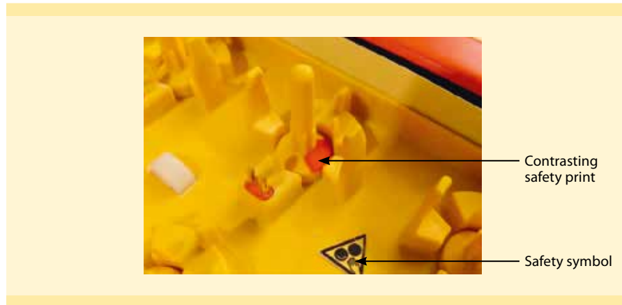
Figure 1: Safety symbol on the Trough of the gentleMACS Octo Dissociator with Heaters. The Sleeves are marked with a contrasting safety print.
