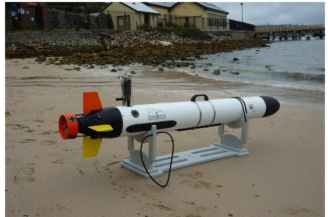
Automated underwater vehicle developed by the Australian Centre for Field Robotics.
