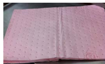
Figure 2: Hazardous chemical absorbent pad
