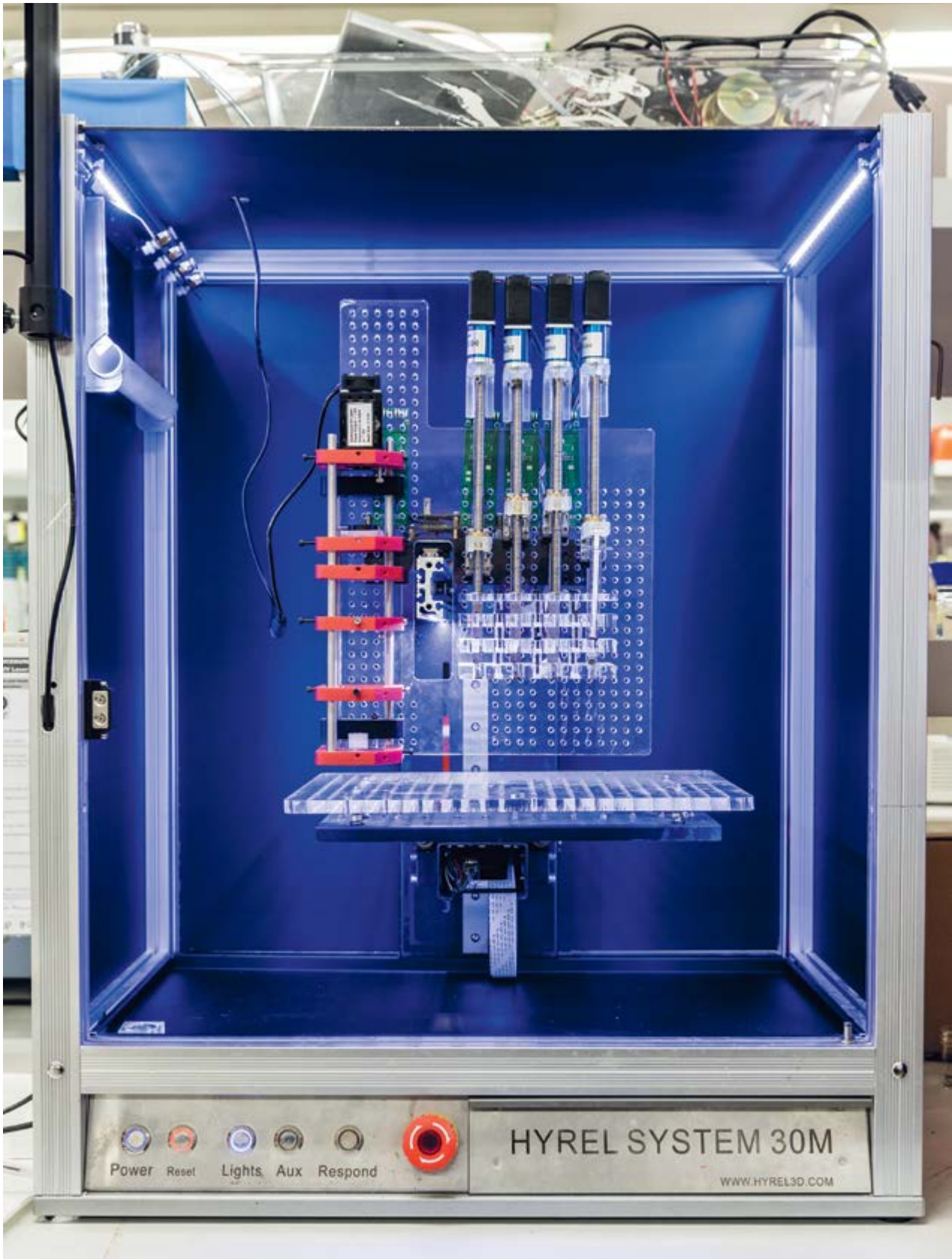
Print me up, Scotty. The ideas that led to 3D printing were coming together in the early 1980s. Zreiqat's team uses this machine to print bone substitute.
