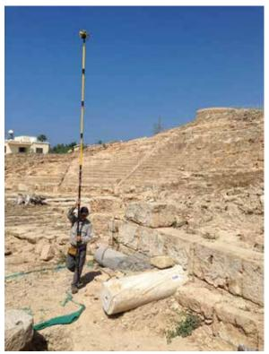
Fig. 4: Surveyor Guy Hazell conducting a pole photograph survey on the site of the ancient theatre.
