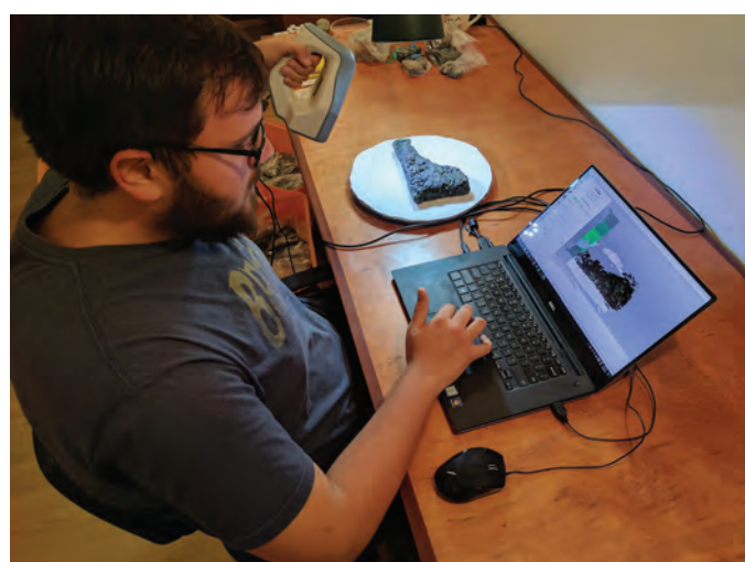
Figure 6: Samuel Martin (University of Arkansas) in July 2017 using a handheld structured light scanner to produce a 3D model of an oxhide ingot quarter (J.W. Lehner).
