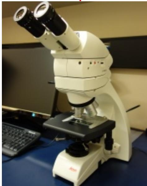
Leica DM750 Optical Microscope
