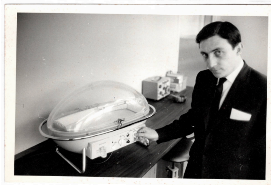
Graham Grant with the first production prototype of the portable premature infant incubator he developed and designed.
