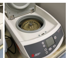
Centrifuges for a variety of uses including cell extract clarification
