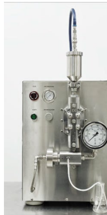
Homogeniser (left) and sonicator (right), for cell lysis
