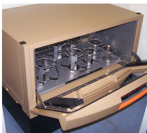
Shaking incubators for bacterial, insect or mammalian cells culture
