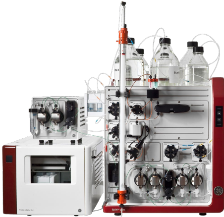
ÄKTA Pure with a size exclusion column and two different affinity columns
