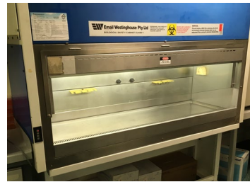
Cell culture cabinet (left) for sterile work with mammalian and insect cells, and microscope (right)
