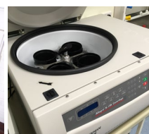
Centrifuges for a variety of uses including cell extract clarification
