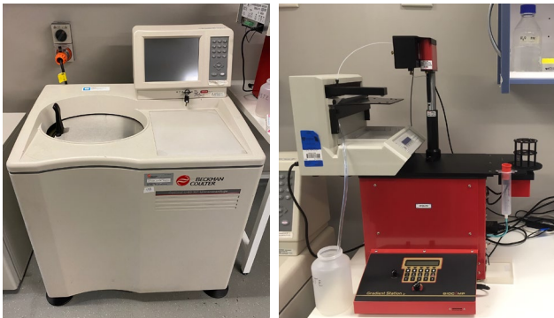
Ultracentrifuge (left) and Gradient Station (right)
