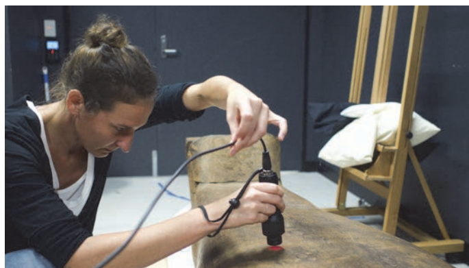
Contactless NIR analysis of pigments on the cedar coffin of the woman Mer-Neith-it-es; 26th Dynasty (664 BC to 525 BC, Saite Period); Saqqara, Lower Egypt (NMR.29.1-2) Nicholson Museum, the University of Sydney
