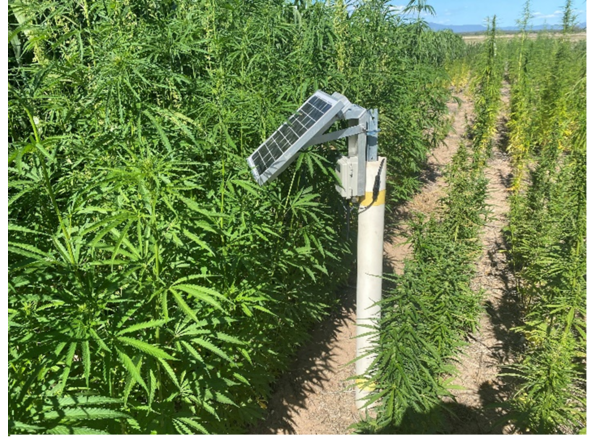
Figure 4: Soil probes used to record soil moisture and temperature for the Low THC Industrial Hemp Trial
