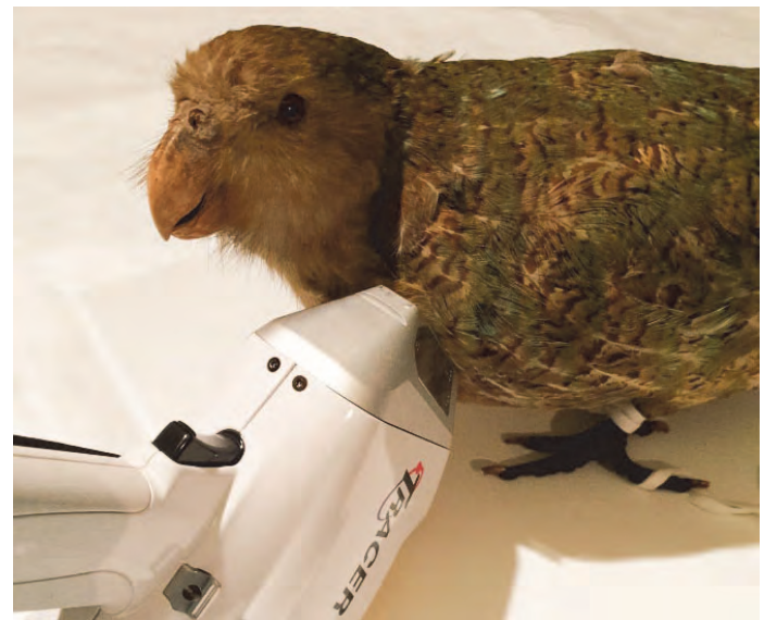
Analysis of Kakapo (NHB.1749) held in the Macleay National History Collection, Sydney University Museums, using a Bruker Tracer 5i portable XRF spectrometer.
