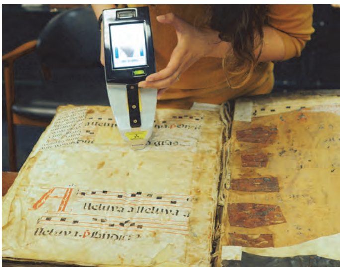
On-site pigment and ink analysis of antiphoner manuscript Add.Ms.413 held in the Rare Books and Special Collections Library, University of Sydney, using the Bruker Tracer 5i.
