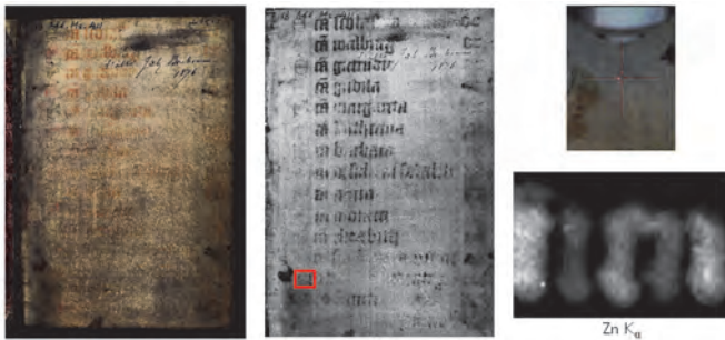
Image of a folio analysed with micro-XRF (left) and an example of its digital alteration (middle), with an area of unreadable text outlined in red. A micro-XRF map of Zn (right) reveals the original text.
