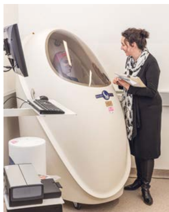
The BodPod measures body fat through air displacement. A smaller version, the PeaPod, is used for babies.
