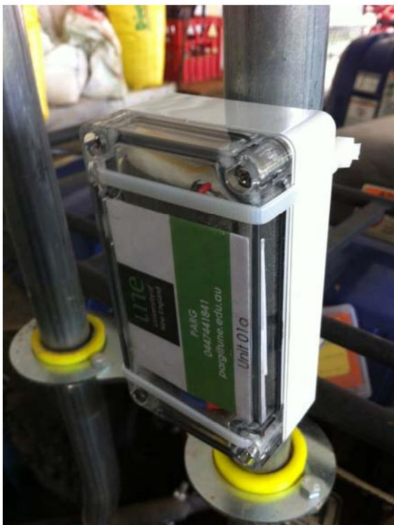
**Figure 1:** GPS unit mounted at the base of the CPD
