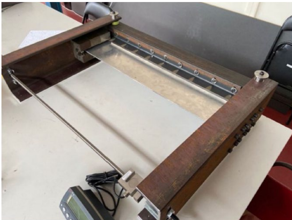
Test rig for plate supported on three edges
