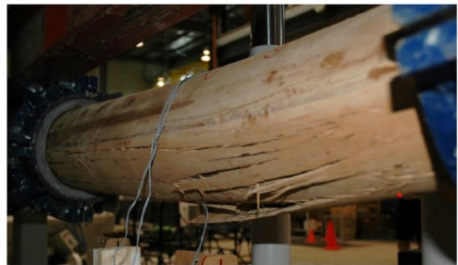
Testing of veneer-based timber circular hollow section beams
