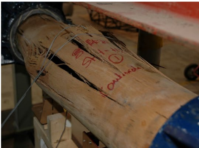
Testing of veneer-based timber circular hollow section beams
