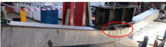
Local buckling of top flange and parts of web
