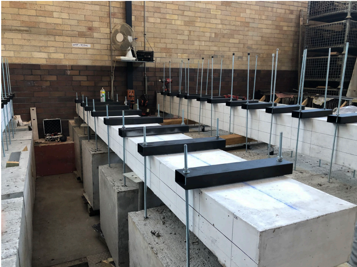
Time-dependent testing of fibre reinforced concrete beams
