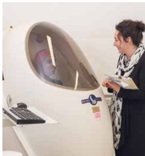
▲ The Bod Pod measures body fat through air displacement. A smaller version is used for babies.
