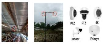
*Figure 1* - The video data collection settings: indoor camera setup (left), outdoor camera setup (middle), and the cameras used for data collection (right).
